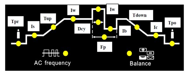
Start left to right. Rotate the red knob to highlight the Parameter to adjust. The yellow light will illuminate to show selection. Push red knob to set parameter value.
