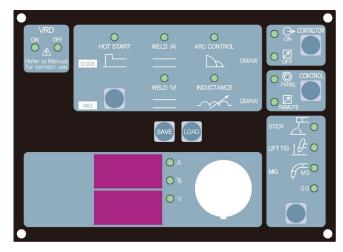
adjustment set Control to Panel (Upper indicator illuminated) and turn encoder knob till 400M/MP reads maximum CV voltage on digital meter. Set Control back to Remote. Full CV Voltage control is now available on the Sky 4HD.
