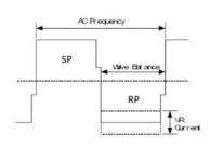
AC Soft includes all the benefits of AC square wave with the addition of maximum puddle control and good wetting action of the weld puddle which helps to overcome surface tension.
