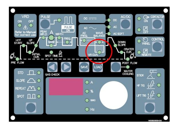
VR-Current is available in all AC modes of operation, the standard AC-Square wave as well as the AC-SOFT modes (AC-sinusoidal and AC-triangle wave).
