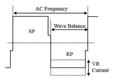
VR-Current along with AC Wave Balance dramatically effects the RP cleaning action.
