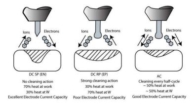
So what actually does the cleaning? It is the positively charge gas ions that bombard the surface of the aluminum to remove the oxide. This action only happens when the AC wave cycle is in reverse polarity. Action is like sand blasting paint off a surface. Cannot weld the aluminum without removing the oxide. The reason is the oxide's melting temperature is way higher than the aluminum being welded. By the time you reach the melting temperature of the oxide the aluminum has melted away.
