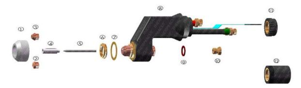
The P22 & P30 Torches have an internal liner. There are two O-Rings inside the torch that seal the liner in the torch. The welding Tips thread into the liner.
