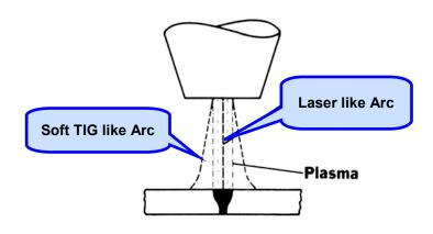
Welding Arc Modes: Soft Tig like Arc or Laser like Arc.
